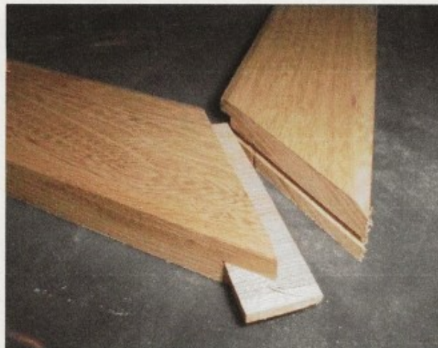
Photo 2 - Spline placed into a groove cut into the miters
