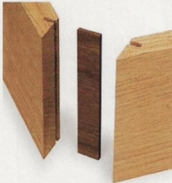
Photo 4 - Splined Miter Joint used in Boxmaking
